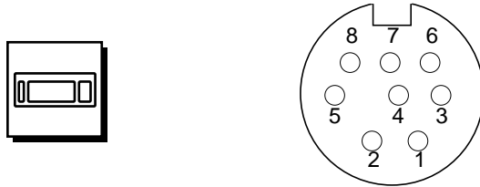
FIGURE B-1 Keyboard/Mouse Connector Pin Configuration
